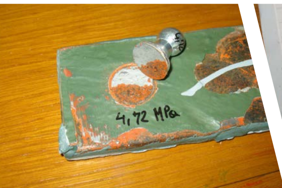
Bridge piece, painted with alkyd paints and lead minium
