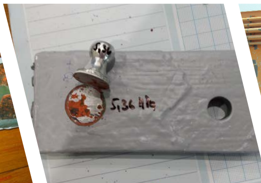
Same piece repainted with MCU
